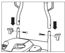
**Step 1** Attach the handle to the frame of the pressure washer. Align holes, insert bolt, and tighten with knob.
